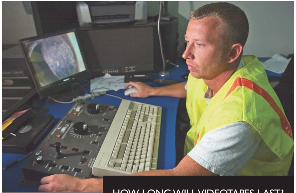
Top left: A map generated by Geomedia GIS software in the a city TV truck shows a neighborhood in which a crew is doing root control work using. Bottom left: A foaming pipeline root control formulation kills roots in the City of Fairfield's sewers. Right: Assistant foreman Jason Turner controls a remote camera as he views live video of sewer lines from the TV truck.
