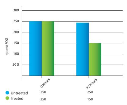
ppm FOG measured using InfraCal® TOG/TPH Analyzer (Model HATR-T2), by Wilks Enterprise, Inc.
